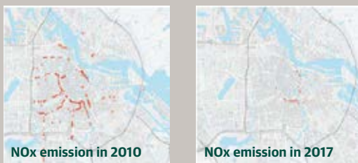
Figure 6. Red dots indicate that the Nitrogen level is exceeding the limit of 40.5µg/m3 (EU directive).
