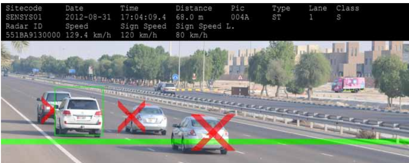
VID – On multi-lane roads there are often several cars on the "report line". A system equipped with SENSYS' in-house-developed VID software makes it possible to fine the right car even when there are several cars on the report line. The speeding car is marked with a green box while cars that are not speeding are marked with a red cross.
